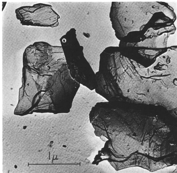
Figure 3. Electron micrograph of the carbon shells of tridymite particles. After diffuse coating with carbon in a vacuum, the tridymite was dissolved away by hydrofluoric acid; specific surface area of this sample of relatively coarse crystals is 7.7 sq. meters/gram ( \times 24,000 )
